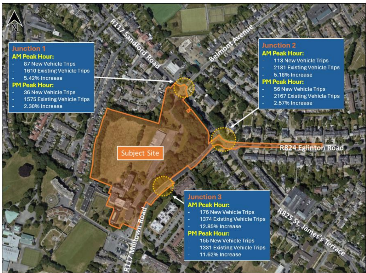
Figure 15.18: Increase in Vehicle Trips Generated Through Key Site Junctions 2043 Do Something – 562 Units
